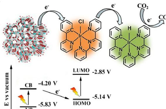
Fig. 8 Z-scheme electron transfer during CO<sub>2</sub> reduction using a NAHN-Tp and [Ir-ppy]. Adapted from ref. 128. © 2020 Published by Elsevier Inc.
