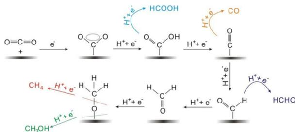
Fig. 6 The proposed reaction mechanism of production of mainly C<sub>1</sub> products by electrochemical CO<sub>2</sub> reduction. Adapted from ref. 100. © 2017 Wiley-VCH Verlag GmbH & Co. KGaA, Weinheim.
