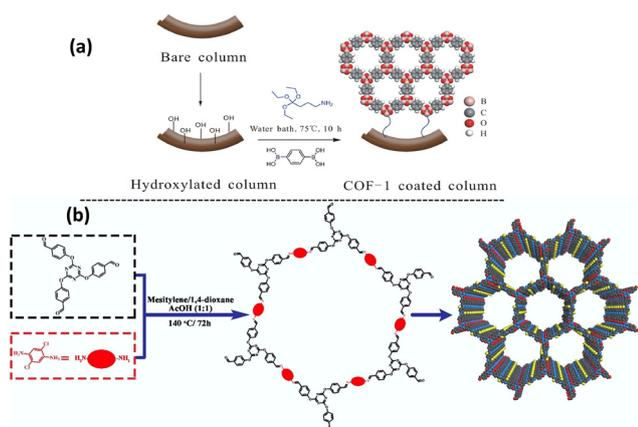
**Fig. 3** A schematic diagram for the development of (a) Boron-based COF and (b) Triazine-based COF. Adapted with permission from ref. 54. Copyright © 2021 Elsevier B.V. All rights reserved; ref. 62. © 2021 Elsevier Ltd. All rights reserved.
