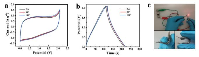
Fig. 6 CV curves at 10 mV s<sup>-1</sup> (a) and GCD profiles at 1 A  $g^{-1}$  (b) of the assembled flexible device at 0–180°. Optical images of the flexible device under different bending conditions (c).
