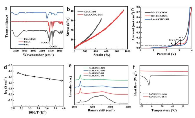
Fig. 2 FTIR spectra of pure PAA, PAAK and PAAK/CMC hydrogel (a), stress-strain curves of PAAK-24 M and PAAK/CMC-24 M (b), LSV curves at a scan rate of 10 mV s<sup>-1</sup> (c), ionic conductivity of the PAAK/CMC-24 M at a temperature from -20 to 70 °C (d), Raman spectra of PAAK/CMC-x (e). DSC thermograms of pure water and 24 M CH<sub>3</sub>COOK in the PAAK/CMC hydrogel (f).
