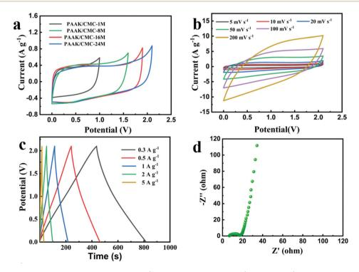
Fig. 3 Voltage windows of PAAK/CMC-1, 8, 16, 24 M at 5 mV s<sup>-1</sup> (a), CV curves from 5 mV s<sup>-1</sup> to 200 mV s<sup>-1</sup> (b), GCD profiles from 0.3 A g<sup>-1</sup> to 5 A g<sup>-1</sup> (c) and EIS (d) of the NG//NG quasi-solid-state supercapacitor with the PAAK/CMC-24 M polyelectrolyte hydrogel.
