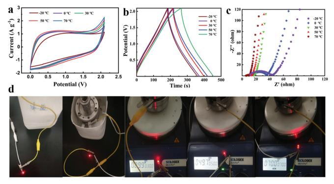
Fig. 5 The NG//NG quasi-solid-state supercapacitor with the PAAK/CMC-24 M polyelectrolyte hydrogel working at different temperatures: CV curves at 10 mV s<sup>-1</sup> (a), GCD curves at 0.5 A g<sup>-1</sup> (b), EIS (c), LED powered (d).
