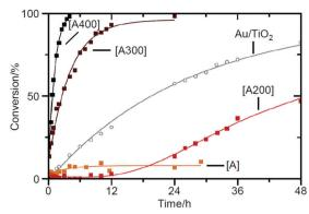
Fig. 6 Kinetic survey of benzyl alcohol dehydrogenation over Au<sub>25</sub>/ SBA-15 materials (1.07 wt% Au) as-synthesized [A] (orange) and calcined at 200 °C [A200] (red), 300 °C [A300] (brown), and 400 °C [A400] (black) and comparison data obtained for Au/TiO2 (gray) (reference from the World Gold Council). Reproduced with permission from ref. 212. Copyright 2015 Elsevier.
