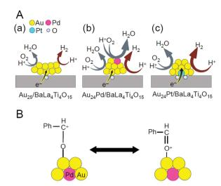
Fig. 38 (A) Proposed structures of  $Au_{24}M/BaLa_4Ti_4O_{15}$  for M = (a) Au, (b) Pd, and (c) Pt during the water-splitting reaction. (B) Resonance structures of carbocationic intermediate. Reproduced with permission from ref. 211 and ref. 244. Copyright 2016 Wiley-VCH and 2019 American Chemical Society
