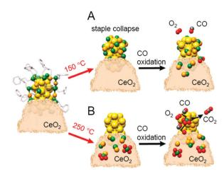
Fig. 19 Evolution of Au<sub>38</sub>(PET)<sub>24</sub>/CeO<sub>2</sub> catalyst structure estimated from EXAFS analyses: catalysts after pre-treatment at (A) 150  $^{\circ}$ C and (B) 250  $^{\circ}$ C and subsequent CO oxidation. Reproduced with permission from ref. 233. Copyright 2020 American Chemical Society.
