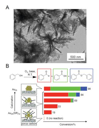
Fig. 5 (A) TEM image of HPCSs. (B) Catalytic performance of  $Au_{25}(SC12)_{18-x}$ HPCSs for aerobic oxidation of benzyl alcohol. Reproduced with permission from ref. 210. Copyright 2014 American Chemical Society
