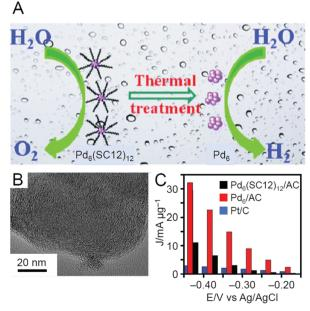
Fig. 30 (A) Schematic of difference in electrochemical reaction before and after thermal treatment of Pd<sub>6</sub>(SC12)<sub>12</sub>/AC (B) HR-TEM images of Pd<sub>6</sub>/ AC. (C) Comparison of the current densities of the HER on the samples at different potentials. Reproduced with permission from ref. 246. Copyright 2017 Royal Society of Chemistry.
