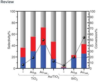
Fig. 11 Catalytic activity of loaded Au<sub>25</sub> and Au<sub>144</sub> NCs (pre-treated at 150 °C) in cyclohexane oxidation. Cyclohexane conversion normalized to the Au loading (except for the blank measurements) (right axis); product distribution (left axis): red, blue, and gray represent cyclohexanol, cyclohexanone, and by-products, respectively. Reproduced with permission from ref. 218. Copyright 2019 Elsevier.
