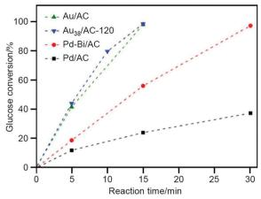
Fig. 7 Glucose conversion vs. time over Pd/AC, Pd-Bi/AC, Au/AC, and Au<sub>38</sub>/AC-120. Reproduced with permission from ref. 213. Copyright 2017
