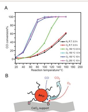
Fig. 16 (A) Reaction temperature dependence of CO conversion over Au<sub>25</sub>(PET)<sub>18</sub>/CeO<sub>2</sub> catalyst after different pre-treatments. Gas hourly space velocity (GHSV) = 7500 mL  $g^{-1} h^{-1}$ . (B) Proposed model for CO oxidation at the perimeter sites of Au<sub>25</sub>(PET)<sub>18</sub>/CeO<sub>2</sub> catalyst. Reproduced with permission from ref. 226. Copyright 2012 American Chemical Society.
