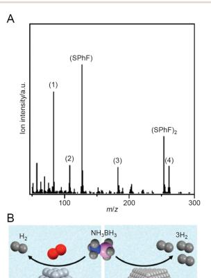
Fig. 25 (A) Typical mass spectrum of the desorbed species from  $[Ag_{44}(SPhF)_{30}](PPh_4)_4$  at 297 °C. The mass peaks of (1) PhF, (2) PPh, (3) PPh<sub>2</sub>, and (4) PPh<sub>3</sub> are fragments of PPh<sub>4</sub> and SPhF, produced by electronimpact ionization. (B) Comparison of H<sub>2</sub> generation from NH<sub>3</sub>BH<sub>3</sub> in the presence of Ag<sub>44</sub> NCs/MPC and Pt<sub>NP</sub>/MPC. Reproduced with permission from ref. 239. Copyright 2015 American Chemical Society.
