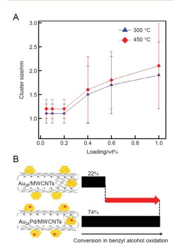
Fig. 4 (A) Dependence of the loading amounts of Au<sub>25</sub> NCs on the Au particle size in Au<sub>25</sub>/MWCNTs. The error bars indicate the size distribution determined by TEM. (B) Catalytic performances of Au<sub>25</sub>/MWCNTs and Au<sub>24</sub>Pd/MWCNTs for benzyl alcohol oxidation. Reproduced with permission from ref. 209. Copyright 2012 American Chemical Society.
