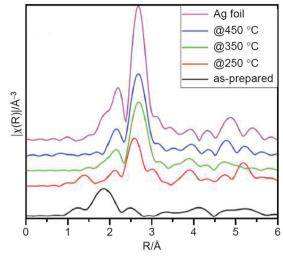
Fig. 15 Ag K-edge FT-EXAFS spectra in R-space for as-prepared and activated Ag<sub>25</sub>/AC catalysts and Ag foil reference. Reproduced with permission from ref. 224. Copyright 2019 Royal Society of Chemistry
