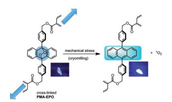
Fig. 3 Application of mechanical stress leads to the emergence of fluorescent anthracene cores presumably *via* cycloreversion with a concomitant singlet oxygen release. Distortion of the endoperoxide bridgehead positions is expected initiate cycloreversion. Inset pictures: appearance of the polymer under irradiation with a hand held-UV lamp at 360 nm, left before (left), and after (right) cryomilling.
