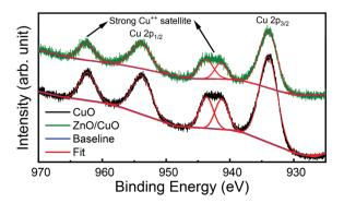
Fig. 6 High-resolution XPS spectra of Cu 2p state in pure CuO nanostructures (black) and ZnO/CuO heterojunction (green).
