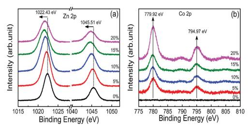
Fig. 4 High-resolution core-level XPS spectra of (a) Zn 2p and (b) Co 2p state in 0-20% cobalt ZnO nanorods.
