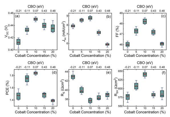
Fig. 10 Statistics of device performance using various cobalt doped ZnO window layer (0-20%). (a) Open circuit voltage  $(V_{OC})$ , (b) short circuit current density ( $J_{SC}$ ), (c) fill factor (FF), (d) power conversion efficiency (PCE), (e) series resistance ( $R_{SH}$ ), and (f) shunt resistance ( $R_{SH}$ ). The solid red circle represents the average values, and the horizontal lines in the box denote the 25th, 50th, and 75th percentile values.
