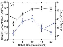
Fig. 8 (a) Conductivity (b) mobility and carrier concentration of 0-20% cobalt doped ZnO.
