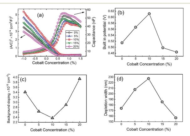
Fig. 14 (a) Capacitance–voltage (C-V) and Mott–Schottky plots of the 0–20% cobalt doped ZnO/CuO heterojunction solar cells. Variation in (b) built-in potential, (c) background doping concentration, and (d) depletion width as a function of cobalt concentration.
