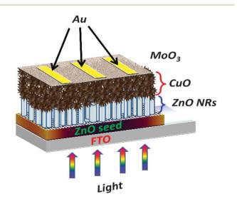
Fig. 1 Schematic design of ZnO/CuO/MoO<sub>3</sub> heterojunction solar cell.
