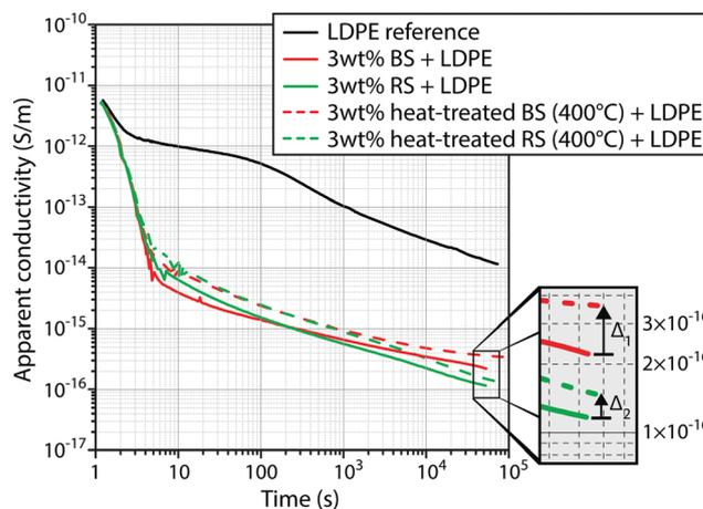
Fig. 3 Apparent conductivity at 60 °C with an electric field of 30 kV mm<sup>-1</sup> for ZnO LDPE composites containing 3 wt% unmodified or heat-treated (400 °C) particles in the shape of rods or balls. The reproducibility of measurements on the composites containing heat-treated particles is shown in Fig. S3 (ESI<sup>†</sup>).
