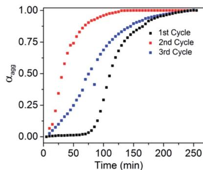
Fig. 6 Variation of  $\alpha_{agg}$  vs. time for living SROP; 2.5% DMAP was used in the first cycle while NDI-1<sub>SP</sub> (NDI-1<sub>mono</sub>/NDI-1<sub>SP</sub> = 34) was used in the 2<sup>nd</sup> and 3<sup>rd</sup> cycles.
