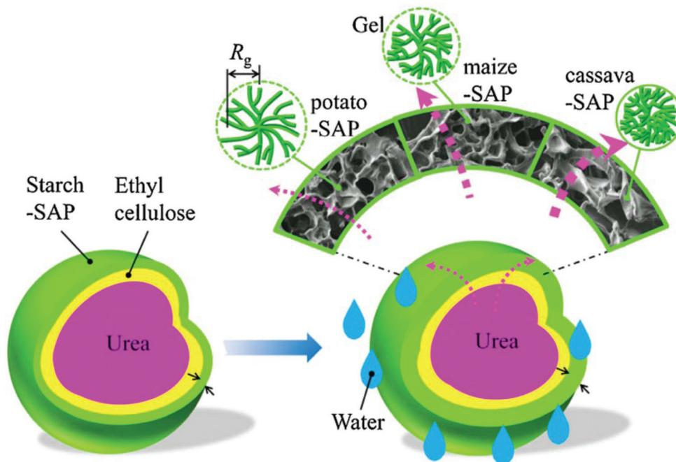
Fig. 11 Schematic representation of the relationship between the slow release behavior of a double-coated SRFH and its starch-SAP characteristics. Reprinted with permission from ref. 45. Copyright (2016) Elsevier.
