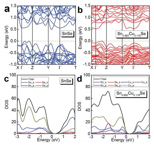
Fig. 7 Calculated band structure of (a) SnSe and (b)  $Sn_{0.882}Cu_{0.118}Se$ , and the calculated density of states (DOS) of (c) SnSe and (d)  $Sn_{0.882}Cu_{0.118}Se$ .
