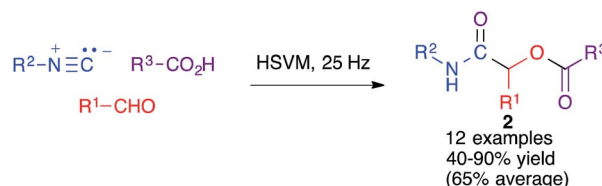
Scheme 2 The mechanochemical Passerini reaction.
