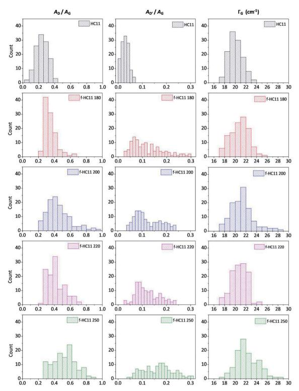
Statistical analysis of the Raman spectra acquired from the HC11 and f-HC11 samples in terms of  $A_D/A_G$ ,  $A_D'/A_G$  and  $\Gamma_G$ .
