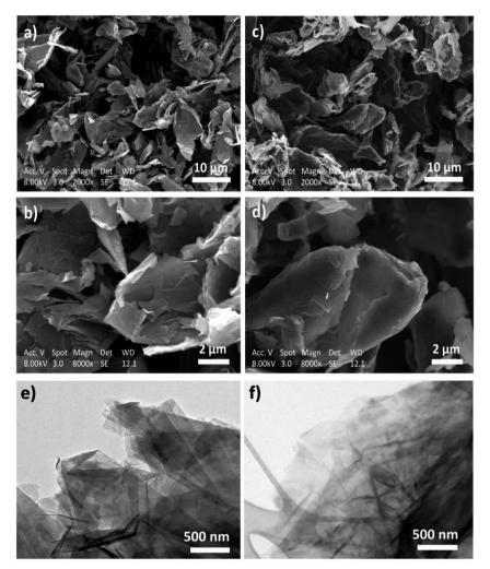
Fig. 7 SEM images of (a) and (b) pristine HC11 and (c) and (d) f-HC11 200; TEM images of (e) pristine HC11 and (f) f-HC11 200.
