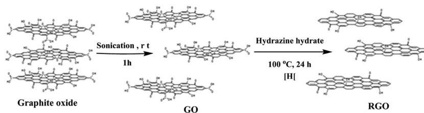
Fig. 3 Schematic representation of reduction of GO to RGO.
