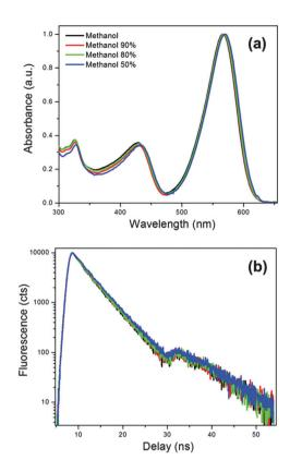
Fig. 6 Absorbance spectra (a) and fluorescence time resolved decay traces (b) recorded for compound 2 in methanol/glycerol mixtures at 25 °C. The corresponding quantum yields were 0.57 (methanol), 0.61 (10% glycerol), 0.63 (20% glycerol) and 0.71 (50% glycerol).
