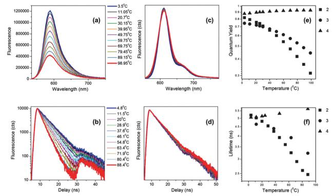
Fig. 3 Fluorescence spectra (a and c) and time resolved fluorescence decays (b and d) of compounds 2 (a and b) and 4 (c and d) in Silicone oil 1000 recorded upon a temperature change between 3.5 and 99 °C. Quantum yields (e) and fluorescence lifetimes (f) recorded for compounds 2, 3 and 4 in Silicone oil 1000 upon a temperature change between 3.5 and 99 °C. Excitation wavelength 560 nm, detection wavelength 589 nm (b) and 612 nm (d)
