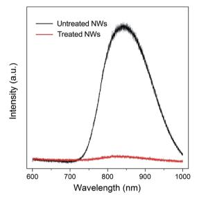
Fig. 3 Photoluminescence (PL) spectra of TiO<sub>2</sub> NW arrays without treatment (black line) and with treatment (red line). The untreated NWs exhibit a strong NIR PL peak centered at about 835 nm, while the PL peak intensity is significantly reduced for the NWs after treatment in H<sub>2</sub>O<sub>2</sub>-NH<sub>3</sub> (aq) solution for 10 min
