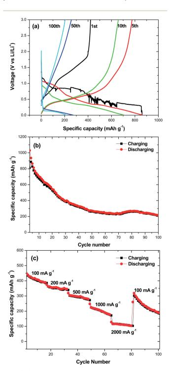
Fig. 8 (a) Charge–discharge curves of the multi-shelled SnO<sub>2</sub> hollow sphere electrode for the 1<sup>st</sup>, 5<sup>th</sup>, 10<sup>th</sup>, 50<sup>th</sup>, and 100<sup>th</sup> cycle at current density of 100 mA g<sup>-1</sup>; (b) the cycling performance of the multi-shelled SnO<sub>2</sub> hollow spheres; (c) charge–discharge curves of the multi-shelled SnO<sub>2</sub> hollow spheres at different current densities.
