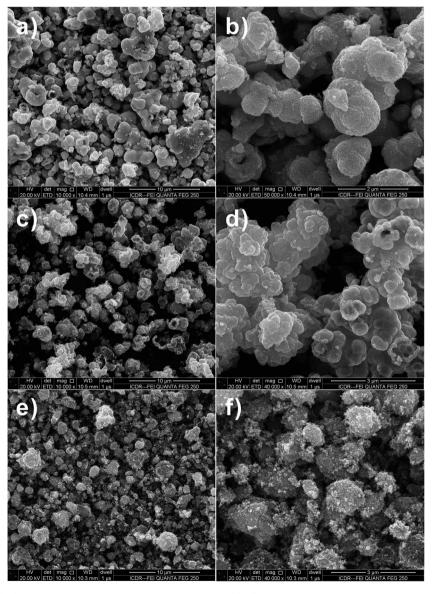
Fig. 1 FESEM images of SnO<sub>2</sub> samples after hydrothermal reaction at 180 °C with 1 : 2 molar ratio of D-glucose and metal salt. (a and b) Na<sub>2</sub>SnO<sub>3</sub>·3H<sub>2</sub>O, (c and d) SnCl<sub>2</sub>·2H<sub>2</sub>O and (e and f) SnCl<sub>4</sub>·5H<sub>2</sub>O.
