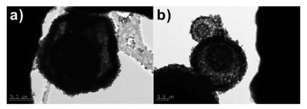
Fig. 7 TEM images of  $SnO_2$  samples after calcination at (a) 700 and (b) 500 °C with 1:1 molar ratio of sucrose and  $SnCl_4 \cdot 5H_2O$ .
