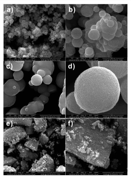
Fig. 3 FESEM images of  $SnO_2$  samples after calcination at 550 °C for 3 h with 1 : 0.4 molar ratio of p-glucose and metal salt. (a and b)  $Na_2-SnO_3\cdot 3H_2O$ , (c and d)  $SnCl_2\cdot 2H_2O$  and (e and f)  $SnCl_4\cdot 5H_2O$ .
