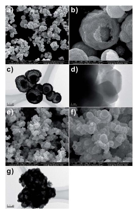
Fig. 5 FESEM and TEM images of  $SnO_2$  samples after calcination at 600 °C for 3 h with 1:1 molar ratio of sucrose and metal salt. (a–d)  $SnCl_4 \cdot 5H_2O$  and (e–g)  $SnCl_2 \cdot 2H_2O$ .
