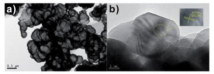
Fig. 4 (a) TEM (b) HRTEM images of  $SnO_2$  samples after calcination at 550 °C for 3 h with 1 : 2 molar ratio of D-glucose and  $SnCl_2 \cdot 2H_2O$ .
