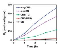
Fig. 21 Hydrogen evolution of S-doped  $g-C_3N_4$  from an aqueous solution of TEA under visible light ( $\lambda > 400$ ) (reproduced from ref. 56, licence number 3767480308846).
