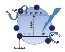
Scheme 6 Photocatalytic charge transfer by co-catalyst loading
