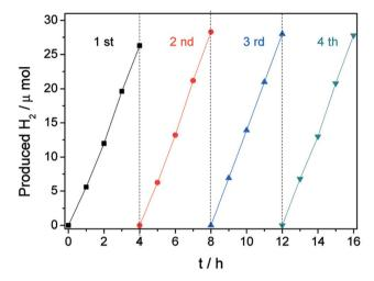
Fig. 23 Long-term  $H_2$  evolution by a Ni/NiO/C<sub>3</sub>N<sub>4</sub> nanocomposite under visible light (reproduced from ref. 96, licence number 3767480083704).
