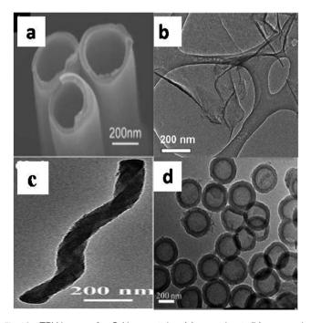
Fig. 10 TEM image of g- $C_3N_4$  nanotubes (a), nanosheets (b), nanorods (c) and hollow nanospheres (d) (reproduced with permission from ref. 20, Copyright American chemical society, 2009, ref. 40 (licence number 3767461234354), ref. 19 (licence number 3767470642681), ref. 44).
