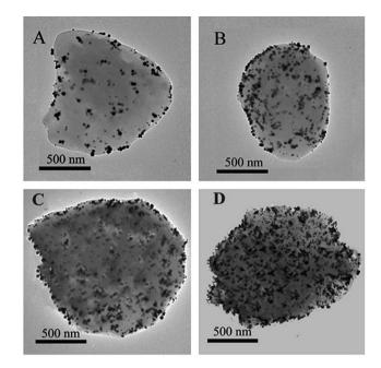
Fig. 11 TEM images of Au/g- $C_3N_4$  samples with different Au loading: (A–D) 20, 60, 80 and 90 wt% (reproduced from ref. 71, licence number 3767470882063).
