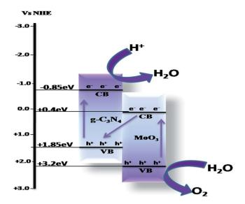
Scheme 5 Photocatalytic charge transfer by a Z-scheme mechanism.
