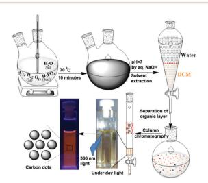
Scheme 1 Preparation and purification of orange-red emitting carbon dots using sucrose and H<sub>3</sub>PO<sub>4</sub>.
