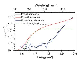
Fig. 3 Absorption spectra of an x=0.6 film before (black) and after (red) white-light soaking for 5 minutes at 100 mW cm<sup>-2</sup>, and after 1 h in the dark (blue). A scaled absorption spectrum of an x=0.2 film (dashed green) is shown for comparison.
