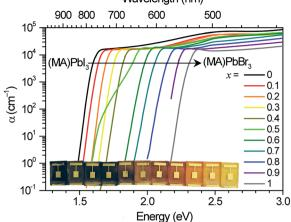
Fig. 1 Absorption coefficient of  $(MA)Pb(Br_xl_{1-x})_3$  measured by diffuse spectral reflection and transmission measurements on thin films and photocurrent spectroscopy of solar cells. Inset: photograph of  $(MA)Pb(Br_xl_{1-x})_3$  photovoltaic devices from x=0 to x=1 (left to right).
