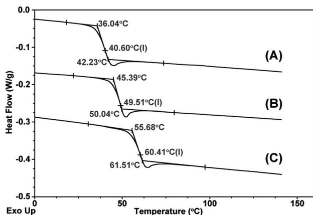
**Fig. 3** DSC thermograms of poly(propylene carbonate) (A) and of PUs prepared by reacting MDI (B and C, entries 9 and 11, respectively) with PPC-diol prepared by feeding 2,6-naphthalenedicarboxylic acid as the chain-transfer agent.
