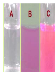
Fig. 2 Naked eye color change with time, (A) only probe, (B) immediately and (C) 30 min after addition of Hg(II) ion in HEPES buffer (1 mM, pH 7.4; 2% EtOH) at 25°C.
