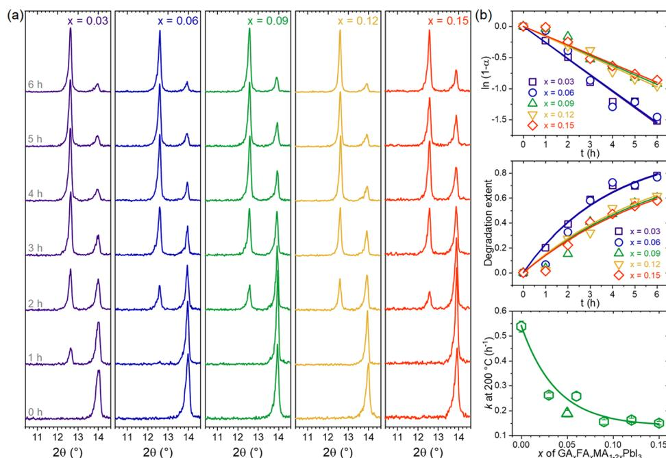
Fig. 6 (a) XRD results of  $\text{GA}_x\text{FA}_x\text{MA}_{1-2x}\text{PbI}_3$  compositions treated for various times at 200 °C. (b) Linear fits used to obtain the thermal degradation rate constants at 200 °C, experimental degradation extent data with reconstructed curves, and composition dependency of the rate constants.
