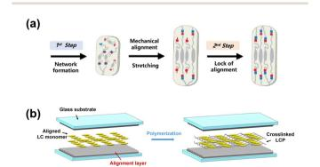
Fig. 3 (a) General schematic of two-step crosslinked method applying mechanical alignment. Reproduced with permission from ref. 26. Copyright 2022 Wiley-VCH. (b) General schematic of one-step crosslinked method applying surface alignment.
