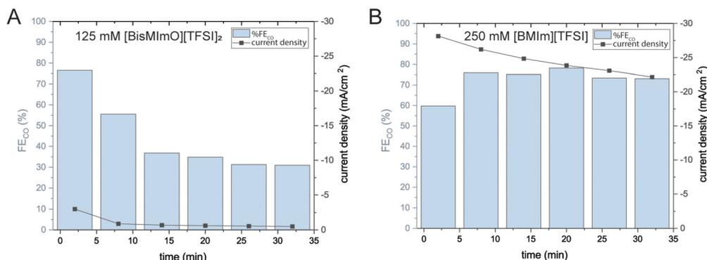
Fig. 3 Representative CA and GC results show that within a few minutes of applying a  $-2.5$  V vs. Ag/Ag<sup>+</sup> potential, the current density and faradaic efficiencies drop for 125 mM [BisMImO][TFSI]<sub>2</sub> (A) but remain relatively stable for 250 mM [BMIm][TFSI] (B). This is due to the formation of (bi)carbonate species at the interface, leading to the growth of a solid precipitate.
