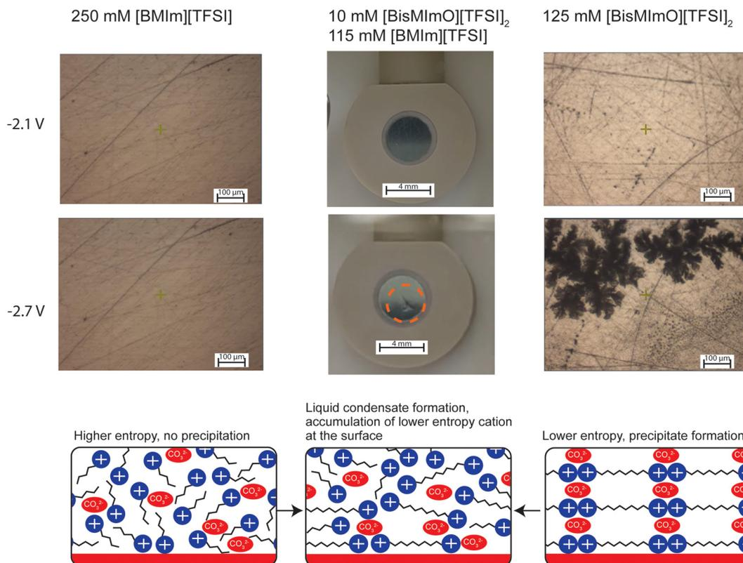
Fig. 7 Ionic liquids with higher entropic penalties of confinement within the double layer form fluid interfaces (left column) while those with lower entropic penalties preferentially accumulate at the interface, which can lead to electrode-blocking precipitate formation (right column). Mixtures of ionic liquids exhibit electrocatalytic behavior that depend on the ion with the lower entropic penalty and can yield liquid–liquid phase separated interfaces (middle column).
