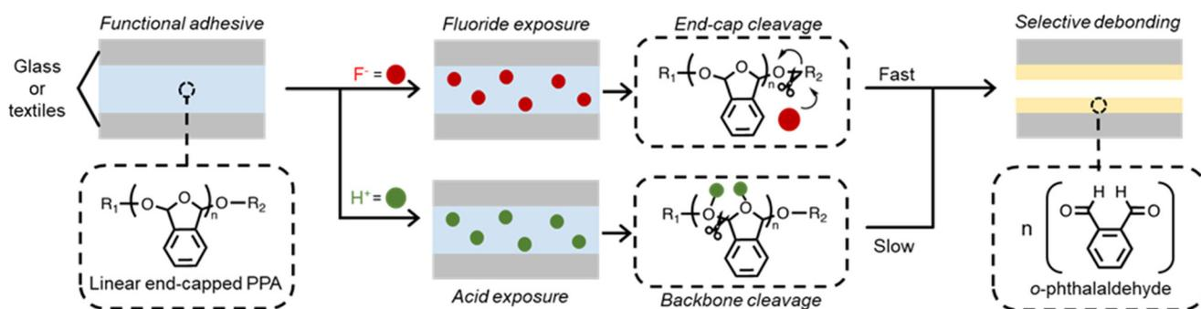
**Fig. 1** On-demand depolymerization of self-immolative PPA and the resulting delamination of surfaces. Two substrates, either glass slides or textiles, are joined with linear PPA, which consists of strategically selected end caps. Upon exposure to a specific chemical stimulus, self-immolative depolymerization rapidly ensues *via* either site-specific or unspecific pathways, thereby releasing the substrates due to structural changes of the material.
