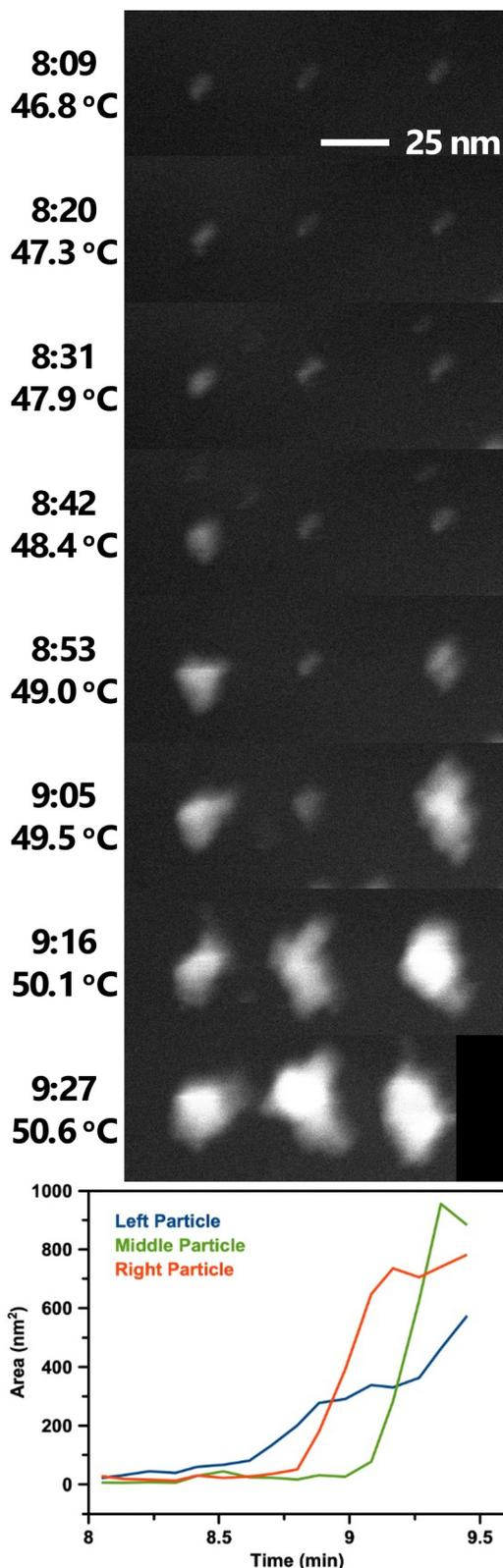
**Fig. 7** Selected STEM images from Movie 2† showing BiOCl formation and growth from BiClLac. Images are spaced ca. 11 s apart with times and temperatures indicated. The black area in the last frame is where the particle clusters drifted near the edge of the field of view and was applied during drift correction. Scale bar applies to all images. Below the images is a plot of the clusters' 2D area over time. Image processing steps for Movie 2 are shown in Movie S1†
