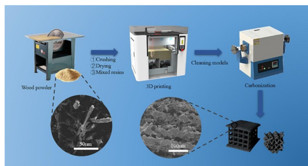
Fig. 12 Schematic diagram of pine resin porous carbon electrode preparation by SLS. 92
