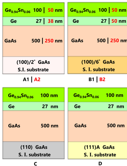
Fig. 1 Cross-sectional schematics of \text{Ge}_{0.94}\text{Sn}_{0.06}/\text{Ge}/\text{GaAs} heterostructures with differently orientated and misoriented semi-insulating (S. I.) GaAs substrates, analyzed in this work: A1 (A2) – 100 (50) nm thick epitaxial \text{Ge}_{0.94}\text{Sn}_{0.06} layer grown on 27 (38) nm Ge buffer with (100)/2° orientation; B1 (B2) – 100 (50) nm thick epitaxial \text{Ge}_{0.94}\text{Sn}_{0.06} layer grown on 27 (50) nm Ge buffer with (100)/6° orientation; C and D – 100 nm thick \text{Ge}_{0.94}\text{Sn}_{0.06} grown on 27 nm Ge buffer with (110) and (111)A orientations, respectively. The \text{Ge}_{0.94}\text{Sn}_{0.06} epilayers are \sim 0.81\% compressively strained.
