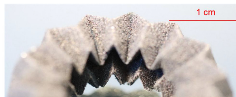
Fig. 1 Printed PM of novel shape with cooling channel.
