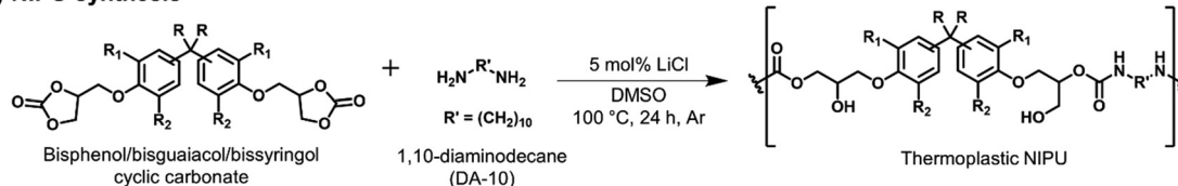
Scheme 1 Synthesis of (a) BGF/BSF using guaiacol/syringol and vanillyl/syringyl alcohol, (b) BGA/BSA using guaiacol/syringol and acetone, (c) diglycidyl ether of bisguaiaicol/bisyringol from respective bisguaiaicol/bisyringol and epichlorohydrin, (d) bisguaiaicol/bisyringol cyclic carbonate from respective diglycidyl ether and \text{CO}_2 , and (e) NIPU using respective bisguaiaicol/bisyringol cyclic carbonate and 1,10-diaminodecane (DA-10).
