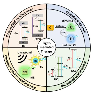
Fig. 1 Schematic illustration of the different mechanisms of light generation with chemi-excitation, NIR-excitation, ultrasound-excitation and X-rayexcitation that support deep-tissue light-mediated therapeutics. (C: chemiluminophore; CL: chemiluminescence; DCL: downconversion luminescence; F: fluorophore; MB: microbubble; ML: mechanoluminescence; NM: nanomaterial; PersL: persistent luminescence; R: radical; RL: radioluminescence; SL: sonoluminescence; and UCL: upconversion luminescence)
