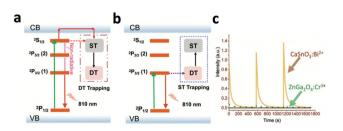
Fig. 11 Schematic illustration of the energy transfer mechanism during (a) high-energy (UV) photon-excited afterglow and (b) low-energy (NIR) photon-excited afterglow. (c) Afterglow decay curves of  $CaSnO_3:Bi^{2+}$  and  $ZnGa_2O_4:Cr^{3+}$ . Reproduced with permission from ref. 108. Copyright 2021, Wiley-VCH Verlag GmbH & Co. KGaA, Weinheim.
