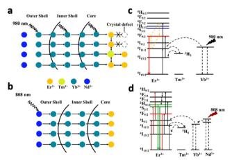
Fig. 13 Schematic illustration of energy migration pathways of NaErF<sub>4</sub>: Yb/Tm@NaYF<sub>4</sub>:Yb@NaNdF<sub>4</sub>:Yb under (a) 980 and (b) 808 nm excitations. Proposed upconversion mechanism for (c) red emission generated under 980 nm laser excitation and (d) green emission under 808 nm laser excitation. Reproduced with permission from ref. 127. Copyright 2019, American Chemical Society
