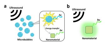
Fig. 23 Schematic illustration of the mechanism of (a) nanomaterialmediated sonoluminescence and (b) ultrasound-excited mechanoluminescence
