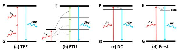
Fig. 8 Schematic illustrations of the energy transfer mechanisms of (a) two-photon excitation (TPE), (b) energy transfer upconversion (ETU), (c) downconversion luminescence (DC) and (d) persistent luminescence (PersL) in NIR-excitable nanomaterials.
