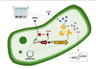
Fig. 11 Process schematic of the bacterial biosensor system used for arsenic detection99 (reproduced from ref. 99; Copyright (2021), with permission from IOP Publishing).
