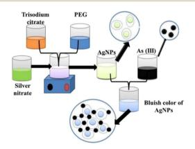
Fig. 6 Functionalised silver nanoparticles as an effective medium towards trace determination of arsenic(III) in aqueous solution<sup>86</sup> (reprinted from ref. 86; Copyright (2019), with permission from Elsevier).
