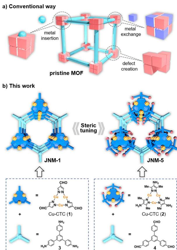
Scheme 1 Schematic illustration of (a) the conventional way for tuning the catalytic performance *via* modification of metal nodes including metal insertion, metal exchange and defect creation; (b) our work *via* steric tuning of metal nodes.
