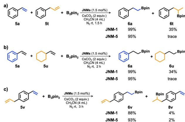
Fig. 4 Competition experiment of JNM-catalyzed hydroboration: (a) reaction conditions: **5a** (0.25 mmol), **5t** (0.25 mmol),  $B_2pin_2$  (1 mmol), 90 min; (b) reaction conditions: **5a** (0.25 mmol), **5u** (0.25 mmol),  $B_2pin_2$  (1 mmol), 2 hours. (c) The chemo-selectivity of JNM-catalyzed hydroboration. Reaction conditions: **5a** (1 equiv.),  $B_2pin_2$  (2 equiv.), 3 hours. All conversions are determined by GC-MS analysis of the reaction mixture.
