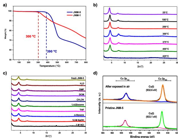
Fig. 2 (a) TGA curves of JNM-5 and JNM-1 (ref. 43) under a  $N_2$  atmosphere. (b) *In situ* variable-temperature PXRD patterns of JNM-5 under a  $N_2$  atmosphere. (c) PXRD patterns of JNM-5 after treatment with different solvents for 3 days. (d) XPS spectra of JNM-5 before and after exposing to air for one month.
