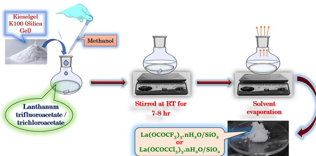
Scheme 2 Silica supported lanthanum trifluoroacetate ( $\text{La}(\text{OCOCF}_3)_3 \cdot n\text{H}_2\text{O}/\text{SiO}_2$ ) and trichloroacetate ( $\text{La}(\text{OCOCCL}_3)_3 \cdot n\text{H}_2\text{O}/\text{SiO}_2$ ) Lewis acid catalyst.
