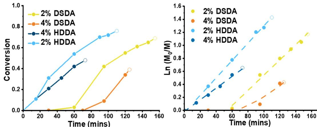
**Fig. 1** Conversion plots (left) and first-order semi-logarithmic kinetic plots (right) for RAFT polymerisations of PBA-DSDA and PBA-HDDA networks. The final point on each data set (open symbol) is the estimated acrylate conversion at the gel point from gel times and through linear regression of the kinetic plots. [BA] : [DDMAT] : [AIBN] : [X] = 100 : 1 : 0.2 : 2 or 4, X = DSDA or HDDA. BA : anisole 1 : 1 v/v; 65 °C, 24 h.
