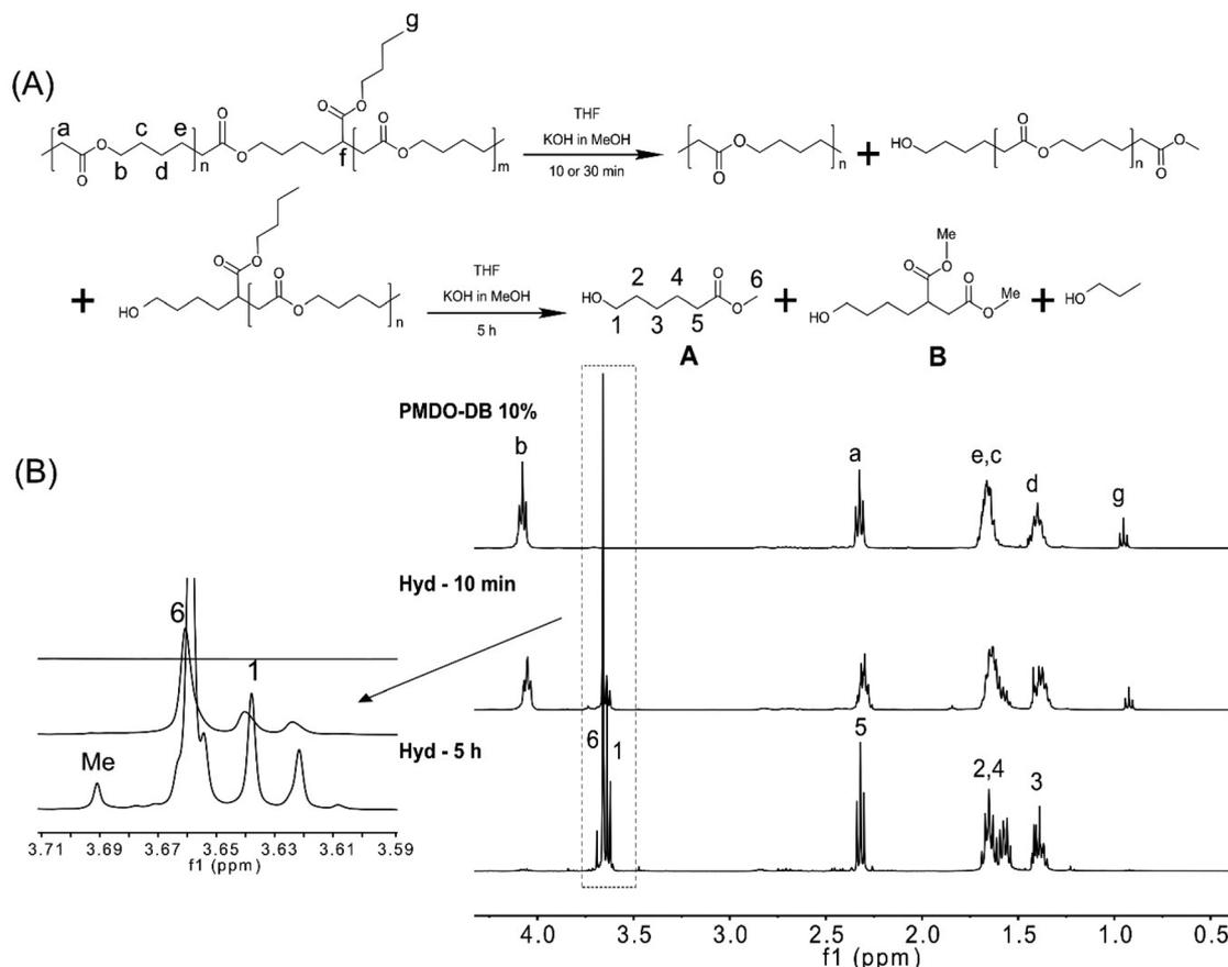
Fig. 5 (A) The hydrolysis mechanism and the proposed hydrolysis products. (B)  $^1\text{H}$  NMR spectra of PMDO-DB 10% and the hydrolysis products of PMDO-DB 10% after 10 min and after 5 h, respectively in  $\text{CDCl}_3$ .
