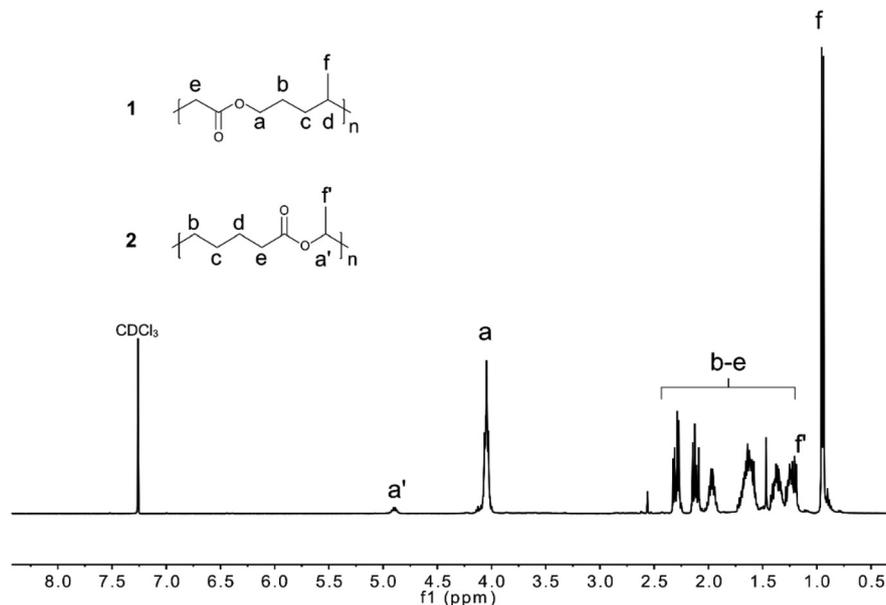
Fig. 3  $^1\text{H}$  NMR spectrum of PMe-MDO in  $\text{CDCl}_3$ .
