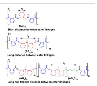
Scheme 4 Increasing distances between ester linkages in AB, AB<sub>x</sub>, and AB<sub>x</sub>C sequences.
