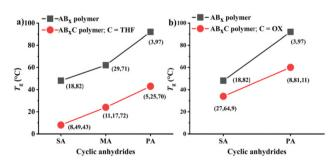
Fig. 8 Comparison of glass-transition temperatures  $(T_q)$  between  $AB_x$ and  $AB_xC$  polymers where (a) C = THF and (b) C = OX, given that (X,Y) =%AB and %AB<sub>x</sub>, respectively, and (X,Y,Z) = %AB, %AB<sub>x</sub> and %AB<sub>x</sub>C, respectively.
