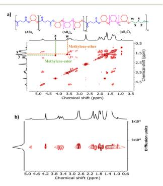
Fig. 7 COSY and DOSY-NMR spectra (600 MHz, CDCl<sub>3</sub>, 30 °C) of the copolymer from ROCOP of SA, CHO and THF using an SA/CHO/THF/ SnOct<sub>2</sub> molar ratio of 50:150:150:1 (Table 2, entry 3).
