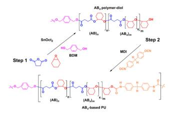
Scheme 2 Synthesis of the AB<sub>x</sub>-based polyurethane.
