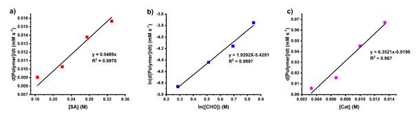
Fig. 4 Plots of initial rates versus (a) SA concentration, (b) CHO concentration and (c) SnOct<sub>2</sub> concentration.
