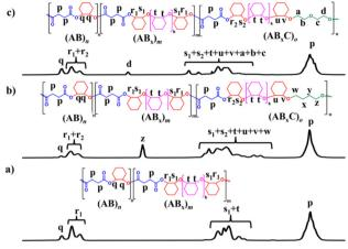
Fig. 6 <sup>1</sup>H NMR spectra (600 MHz, CDCl<sub>3</sub>, 30 °C) of (a) AB<sub>x</sub> copolymer (Table 1, entry 6, for comparison); (b)  $AB_xC$  copolymer; C = THF (Table 2, entry 4); and (c)  $AB_xC$  copolymer; C = OX (Table 2, entry 9).
