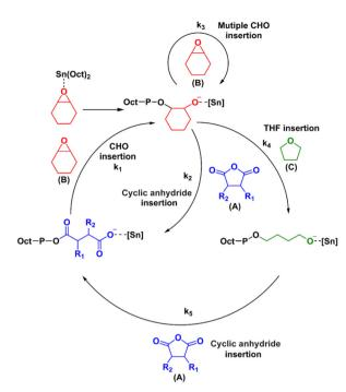
Scheme 3 Proposed mechanism for the formation of AB<sub>x</sub> and AB<sub>x</sub>C poly(ether-ester) from ROCOP of cyclic anhydrides (A), CHO (B) and THF
