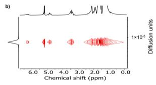
Fig. 5 (a) <sup>1</sup>H NMR and (b) DOSY spectra (600 MHz, CDCl<sub>3</sub>, 30 °C) of poly(ester-ether)-b-PLA.
