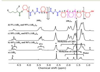
Fig. 2  $\,^{1}$ H NMR spectra (600 MHz, CDCl<sub>3</sub>, 30 °C) of the copolymer from ROCOP of SA and CHO having different AB and AB<sub>x</sub> components.
