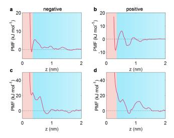
Fig. 3 The tendency for free and bound water electrosorption at electrodes. Potential of mean force (PMF) of water under negative polarization (a) and positive polarization (b) in [Emim][TFSI] as a function of distance from the electrode. PMF of bound water under negative polarization (c) and positive polarization (d) in [Emim][TFSI] as a function of distance from the electrode. The pink-shaded region is considered as the interfacial region (z < 0.35 nm).
