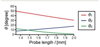
Fig. 5 The tip oscillation angle of the first (red), second (blue), and third (green) eigenmodes,  $\theta_i$  = arctan  $|A_v/A_l|$ , for the properties listed in Table 1 while varying the probe length.  $\theta_1$  is relatively close to 90° (normal to the surface).  $\theta_2$  and  $\theta_3$  are relatively close to 0° (parallel to the surface).
