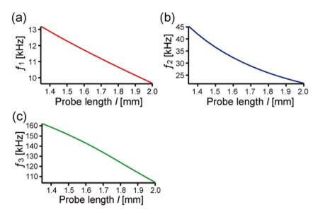
Fig. 3 The first three eigenfrequencies calculated by using the properties listed in Table 1 while varying the probe length. (a) The first eigenfrequency,  $f_1$ . (b) The second eigenfrequency,  $f_2$ . (c) The third eigenfrequency,  $f_3$ .
