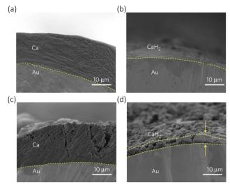
Fig. 3 Cross-section of Au electrodes during calcium plating/stripping in Ca(BH<sub>4</sub>)<sub>2</sub>/tetrahydrofuran. (a) First plating. (b) First stripping. (c) Tenth plating. (d) Tenth stripping. Reproduced with permission from ref. 49, copyright 2017 Nature Springer.
