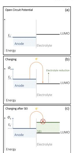
Fig. 2 Energy diagrams of the metallic anode SEI formation. The anode's chemical potential is regarded as its Fermi energy of the anode  $(E_f^-)$ : (a) shows the open circuit voltage at a thermodynamic equilibrium; (b) demonstrates the shift in Fermi level when charged and (c) illustrates the energy level shift with the formation of the SEI
