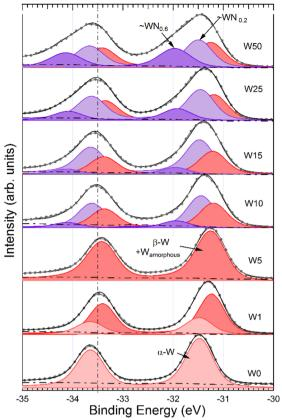
Fig. 5 W4f spectra for W thin film growth in reactive gas mixtures with N<sub>2</sub> (%): 0, 1, 5, 10, 15, 25, and 50. With the progressive enhancement of  $N_2$ , we identified different W-based phases:  $\alpha$ -W,  $\beta$ -W, amorphous W, WN<sub>0.2</sub>, and  $WN_{0.6}$
