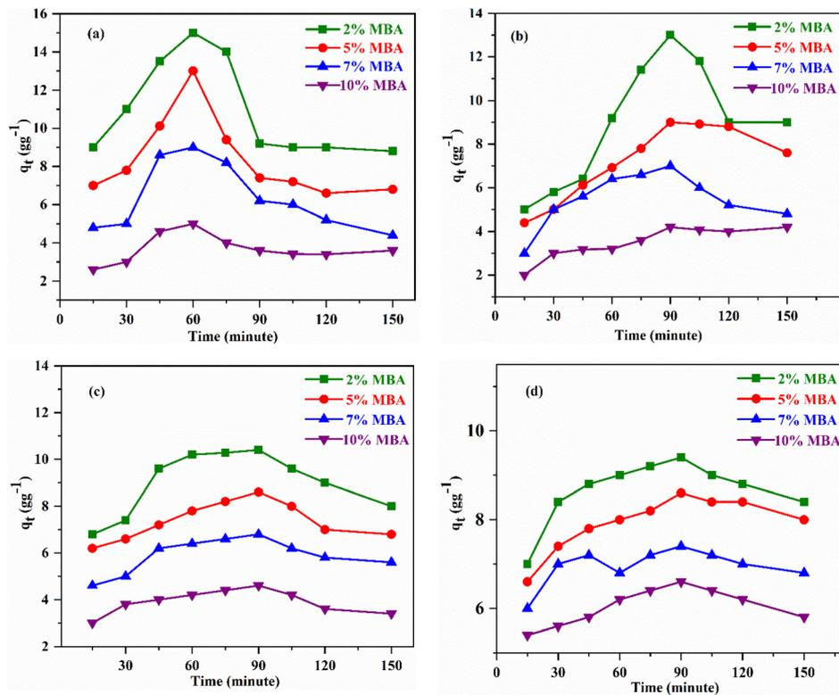
Fig. 5 Adsorption of (a) diesel, (b) petrol, (c) toluene, and (d) petroleum ether by poly(EHA)-*cl*-C<sup>h</sup> with respect to time at 25 °C.
