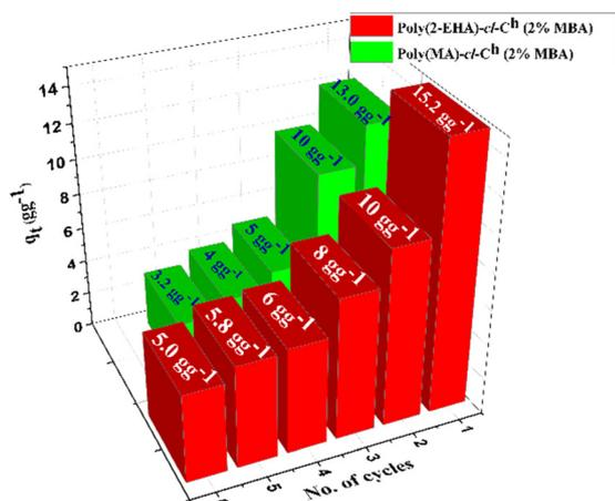
**Fig. 9** Reusability studies of poly(EHA)-*cl*-C<sup>h</sup> (2% MBA) and poly(MA)-*cl*-C<sup>h</sup> (2% MBA) in diesel oil.**Table 4** Adsorption capacities of poly(EHA)-*cl*-C<sup>h</sup> (2% MBA) and poly(MA)-*cl*-C<sup>h</sup> (2% MBA) in the diesel–brine water system
