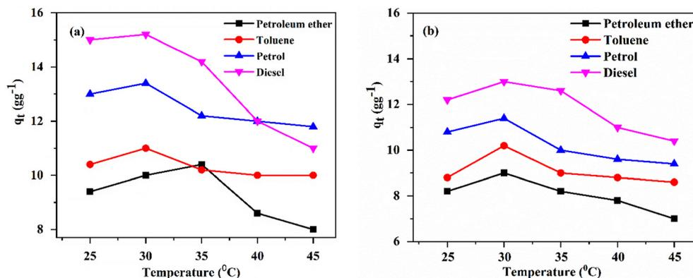
Fig. 7 Adsorption with respect to temperature by (a) poly(EHA)-*cl*-C<sup>h</sup> (2% MBA) and (b) poly(MA)-*cl*-C<sup>h</sup> (2% MBA) at 60 min.
