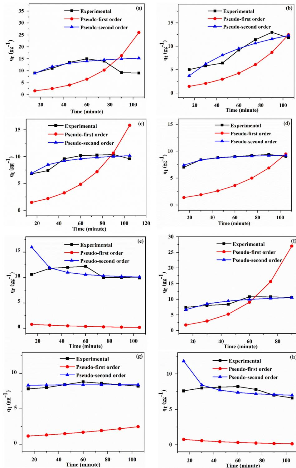
**Fig. 8** Compiled kinetic models of poly(EHA)-*cl*-C<sup>h</sup> (2% MBA) for sorption of (a) diesel, (b) petrol, (c) toluene, and (d) petroleum ether, and poly(MA)-*cl*-C<sup>h</sup> (2% MBA) for sorption of (e) diesel, (f) petrol, (g) toluene, and (h) petroleum ether.
