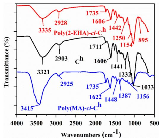
Fig. 1 FTIR spectra of C<sup>h</sup>, poly(EHA)-*cl*-C<sup>h</sup> and poly(MA)-*cl*-C<sup>h</sup>.
