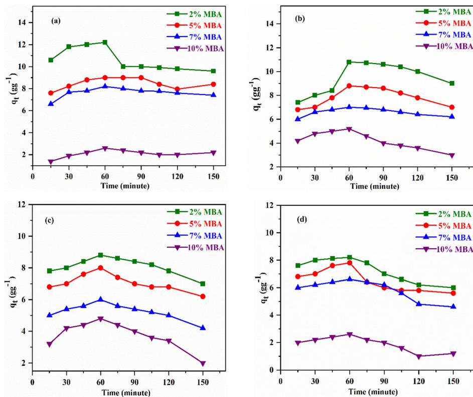
Fig. 6 Adsorption of (a) diesel, (b) petrol, (c) toluene, and (d) petroleum ether by poly(MA)-*cl*-C<sup>h</sup> with respect to time at 25 °C.
