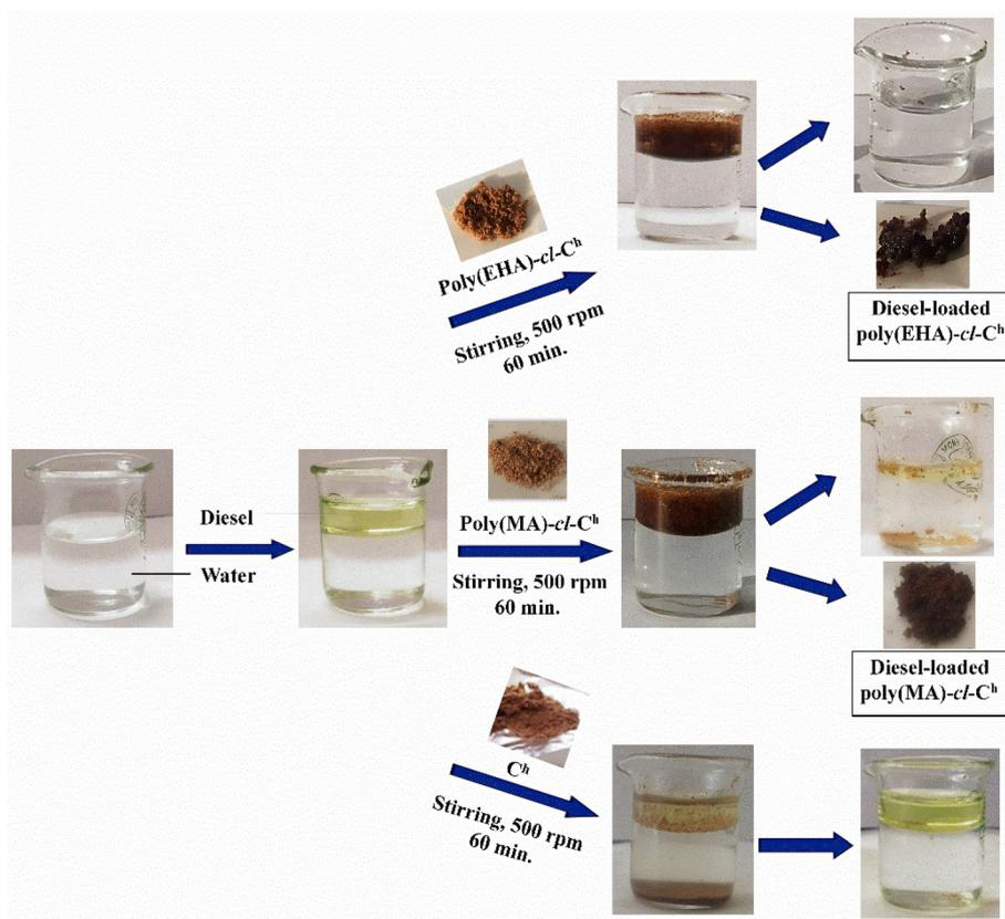
**Scheme 1** Adsorption of oil from oil–water emulsions with poly(EHA)-*cl*-C<sup>h</sup>, poly(MA)-*cl*-C<sup>h</sup>, and pristine C<sup>h</sup>, the backbone.
