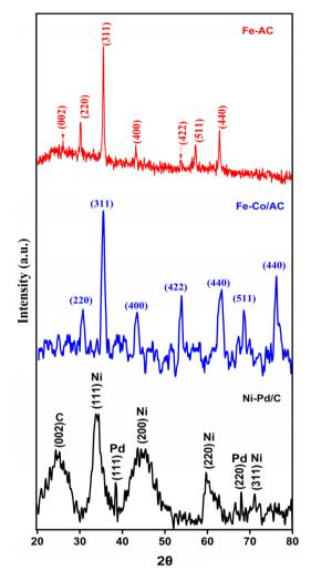
Fig. 2 The XRD spectrum of AC-Fe (red); CoFe-AC (blue); and Ni-Pd/C (black) catalysts with the respective planes.
