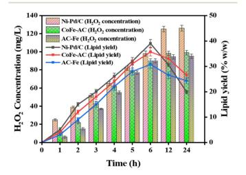
Fig. 8 Algal lipid yield obtained under different H<sub>2</sub>O<sub>2</sub> concentrations produced by Ni-Pd/C, CoFe-AC, and AC-Fe catalysts.
