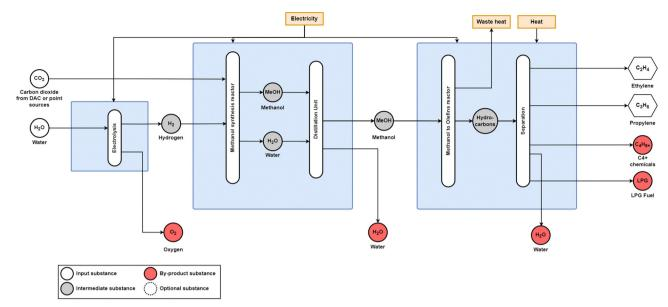
Fig. 13 Power-to-methanol-to-olefins process diagram. Methanol synthesis occurs over a CuOZnO/Al<sub>2</sub>O<sub>3</sub> catalyst and the MTO reactor uses the SAPO-34 catalyst. Adapted from Jiang et al. 25 and Dimian and Baldea. 75
