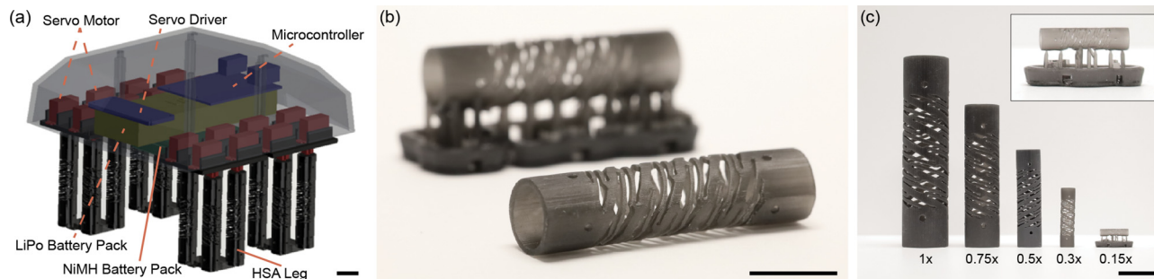
Fig. 1 3D printed HSAs for untethered soft robots. (a) A CAD rendering of the untethered soft robot shows the overall assembly, including four HSA-based legs, 16 servo motors, and on-board electronics and batteries enclosed within the robot's shell. (b) Photographs of a miniature HSA (0.3 \times scaling) show the part before (out-of-focus, in the background) and after processing (foreground). (c) 3D printed HSAs are shown at 1 \times , 0.75 \times , 0.5 \times , 0.3 \times , and 0.15 \times scalings. The inset in the upper right corner is a magnified view of the 0.15 \times HSAs, which can be printed but with supports that are difficult to remove without damaging the HSA. Scale bars are 20 mm (a and c) and 10 mm (b).
