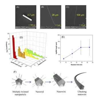
SEM images illustrating the effect of reaction time 4 h (A), 8 h and (B), 24 h (C) and length distribution of the AgNWs (D) and average size of the AgNWs (E) with respect to reaction time and (F) schematic illustration of ultralong nanowire formation.
