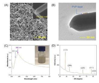
Fig. 1 SEM (A), TEM (B), UV-Vis (C) and XRR (D) characterization results of the AqNWs.
