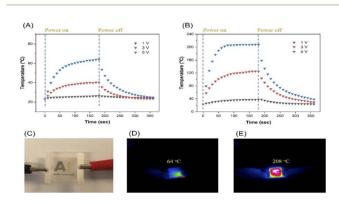
Fig. 10 Time-dependent temperature profile of AgNW films (A) shorter nanowires and (B) longer nanowires, (C) macro photograph of the AgNW film based thermal heater, thermal camera images of the AgNW film at 5 V (D) shorter nanowires and (E) longer nanowires.
