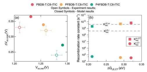
Fig. 4 Voltage loss analysis. (a) Measured voltage losses for the three devices in closed circles and the results of the non-radiative voltage loss model in open circles. (b) Calculated rate constants of radiative and non-radiative recombination from the CT state for the three devices as a function of the free energy difference between the LE and CT state (the values of the free energies of the CT and LE state are the one in Table S7, ESI†).
