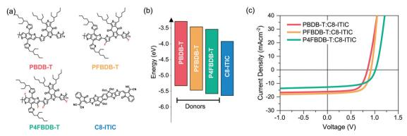
Fig. 2 Materials and device performances. (a) chemical structure of the three donor polymers PBDB-T, PFBDB-T and P4FBDB-T and the acceptor C8-ITIC, (b) energy level (HOMO and LUMO) of the different donors and the acceptor, as estimated using cyclic voltammetry measurement according to results in ref. 12 and Table S4 (ESI†). (c) Current density voltage characteristics under simulated solar irradiation for the three devices considered in the study.
