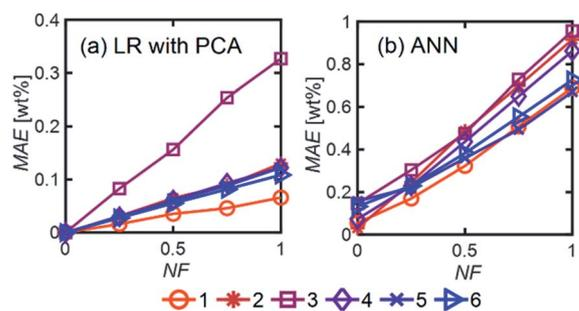
Fig. 7 MAE (averaged over all components) as a function of NF for (a) LR with PCA and (b) ANN over mixtures with different numbers of components and using  $N_{\text{train}} = 400$ . For ANN, we used 1 hidden layer with 12 neurons with the 'relu' activation function and a batch size of 60.
