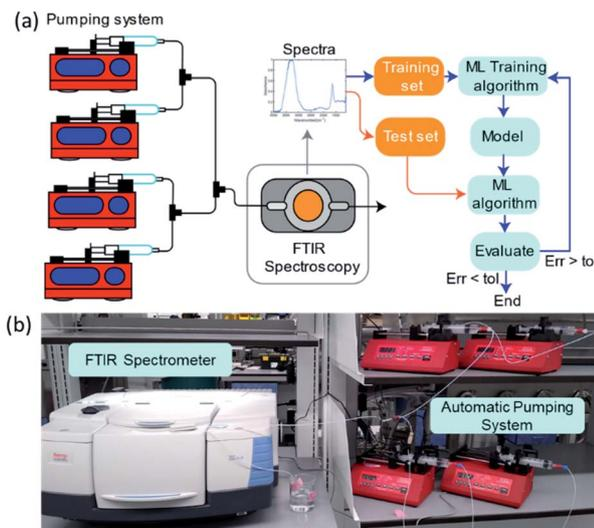
**Fig. 9** (a) A schematic illustration of the experimental set-up with four pumps. Components are mixed using T-mixers and then delivered to a transmission flow cell, with ZnSe windows, inside the sample compartment of an FTIR spectrometer. The collected spectra are used to train and test the ML model for concentration prediction. (b) Photograph of the pumping system and FTIR spectrometer.
