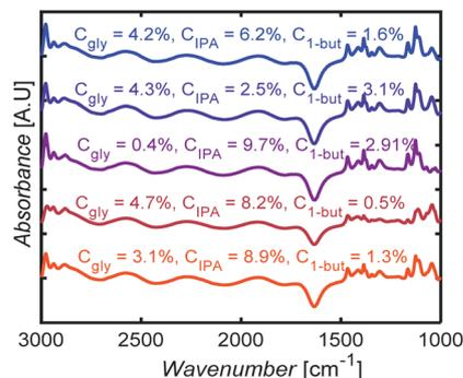
**Fig. 10** FTIR spectral measurements for glycerol (gly), isopropanol (IPA), and 1-butanol (1-but) mixtures at different mass concentrations,  $C_{\text{gly}}$ ,  $C_{\text{IPA}}$ ,  $C_{\text{1-but}}$ , respectively.
