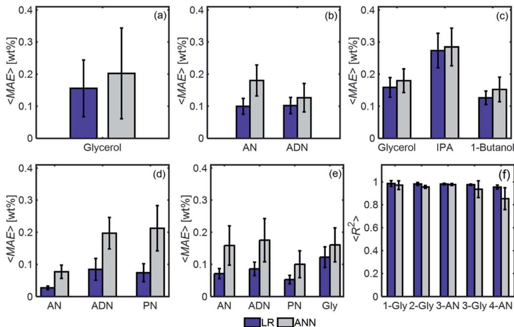
Fig. 11 (a–e)  $\langle \text{MAE} \rangle$  [wt%] for 1-, 2- and 3-component mixtures, for ANN and LR models. Over 200 models were evaluated, each with a different train/test subset, and the average MAE is reported. (f)  $\langle R^2 \rangle$  for the four mixtures considered.
