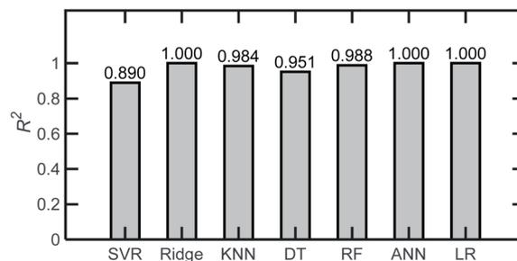
Fig. 4 Coefficient of determination,  $R^2$  averaged over the 6 components for different ML algorithms and for a base case of AN, ADN, and PN in water, applying PCA as a preprocessing step. Two hundred simulated spectra and an 80–20% train-test partition were used in the analysis.
