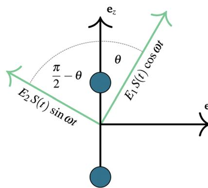
Fig. 1 Diagram of the H<sub>2</sub><sup>+</sup> molecule under an elliptically polarized field. The field can be understood as two perpendicular linearly polarized fields with different amplitudes that differ in phase by  $\pi/2$ .
