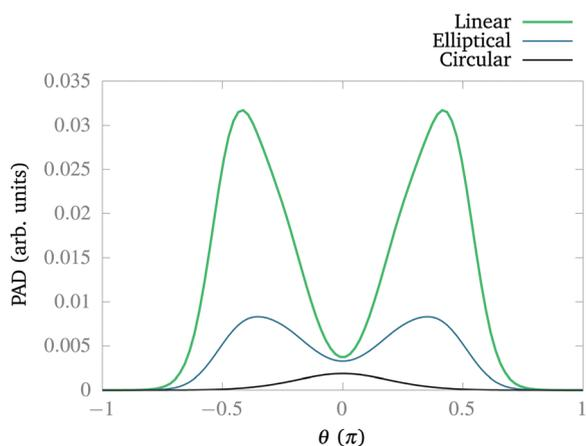
Fig. 6 Angular distribution of the dissociating fragments for linear, elliptical, and circular polarization after 10 fs of simulation. The integral is taken from  $R_1 = 6a_0$  to  $R_2 = 10a_0$ . We use  $E_1 = 0.02$  a.u. and  $E_2 = 0.01$  a.u. for the elliptically polarized case,  $E_1 = 0.04$  and  $E_2 = 0$  for the linearly polarized case, and  $E_1 = E_2 = 0.02$  a.u. for the circularly polarized case. In all these cases, we set  $\omega = 0.1$  a.u.
