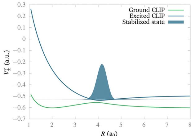
Fig. 2 Ground and excited light-induced potentials created by a strong field of circular polarization (CLIPs) with  $\omega = 0.1$  a.u. and  $E_1 = E_2 = 0.02$  a.u. as a function of the internuclear distance. The curves do not depend on  $\theta$ . Also shown is the ground vibrational wavefunction in the excited CLIP. Note that the CLIPs exhibit bond hardening, bond softening and an avoided crossing for all values of the angle.
