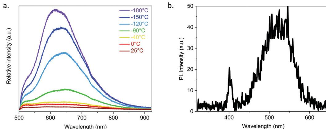
Fig. 3 Photophysical properties of  $[\text{Ag}_2(1,3\text{-BDT})]_n$ : (a) temperature-dependent solid state emission spectra ( $\lambda_{\text{ex}} = 410 \text{ nm}$ ) and (b) second harmonic generation response with incident beam at  $\lambda_{\text{ex}} = 800 \text{ nm}$  and RT.
