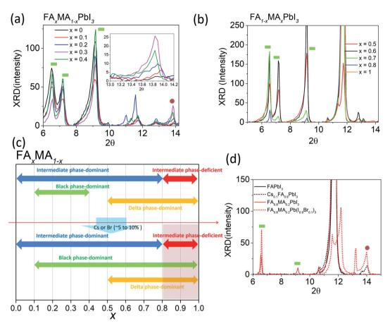
Fig. 4 XRD results for wet films consisting of glass/perovskites ( $FA_xMA_{1-x}PbI_3$ ) at (a) x = 0, 0.1, 0.2, 0.3, and 0.4 and (b) x = 0.5, 0.6, 0.7, 0.8, and 1. (c) Different phases with respect to x. (d) XRD results for wet films with/without Cs or Br.
