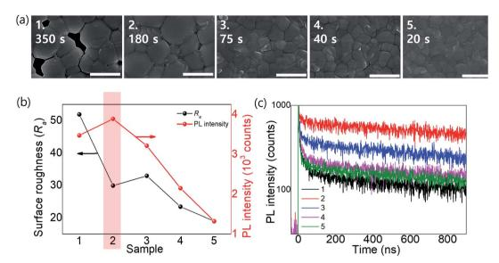
Fig. 5 (a) SEM images, (b)  $R_a$  and PL intensity values, and (c) TRPLs of perovskite films of Rb<sub>0.03</sub>Cs<sub>0.05</sub>(FA<sub>0.83</sub>MA<sub>0.17</sub>)<sub>0.92</sub>Pb(I<sub>0.83</sub>Br<sub>0.17</sub>)<sub>3</sub> with different  $t_{\rm evap}$  values (20–350 s).
