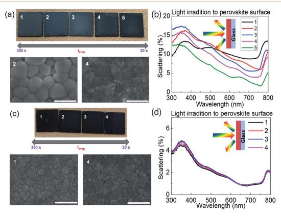
Fig. 1 (a and c) SEM images and (b and d) light-scattering spectra for (a and b)  $FA_{0.8}MA_{0.2}Pb(I_{0.9}Br_{0.1})_3$  and (c and d) MAPbI<sub>3</sub> on glass with different  $t_{\rm evap}$  values.
