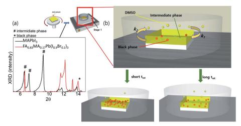
Fig. 2 (a) XRD of wet films (before annealing) for MAPbI<sub>3</sub> and  $FA_{0.8}MA_{0.2}Pb(I_{0.9}Br_{0.1})_3$ ; (b) illustrations of  $t_{ret}$ -sensitive films at stage 1.
